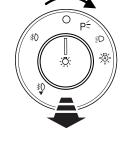
illuminate when the fog lamps have been turned on. The fog lamps will not operate when the high beams are active.
